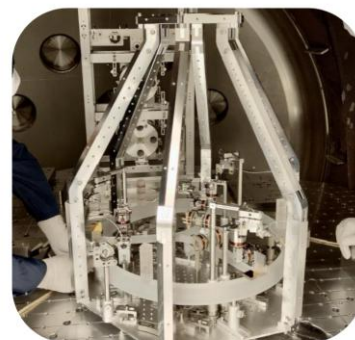
C-6D undergoing installation at MIT LASTI facility
