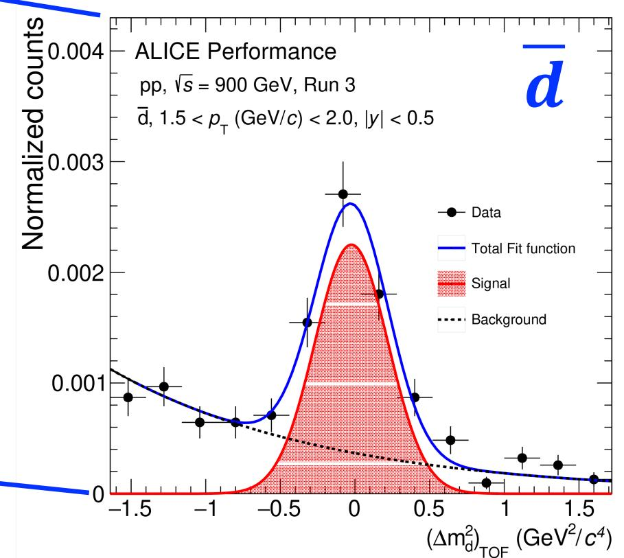
$$m_{TOF} = p \sqrt{\left( \frac{t_{TOF} - t_0}{L} \right)^2 - 1}$$
