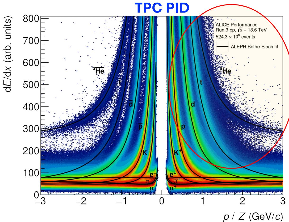
Low momentum ( $p_T < 1\text{--}3$  GeV/c) PID via energy loss in the gas
