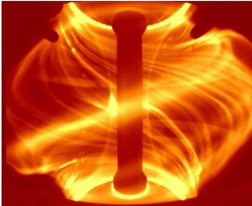
High-speed video image of the MAST plasma obtained at the start of an Edge Localized Mode.
