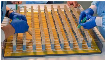
Flat cables positioning before mounting on the back plane
