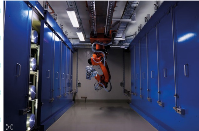
Storage shelves for ISOLDE and CERN-MEDICIS targets after their operation, showing the robot for remote handling. Image credit: Yury Gavrikov.
