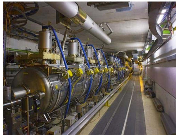
LHC Superconducting RF accelerating cavities
