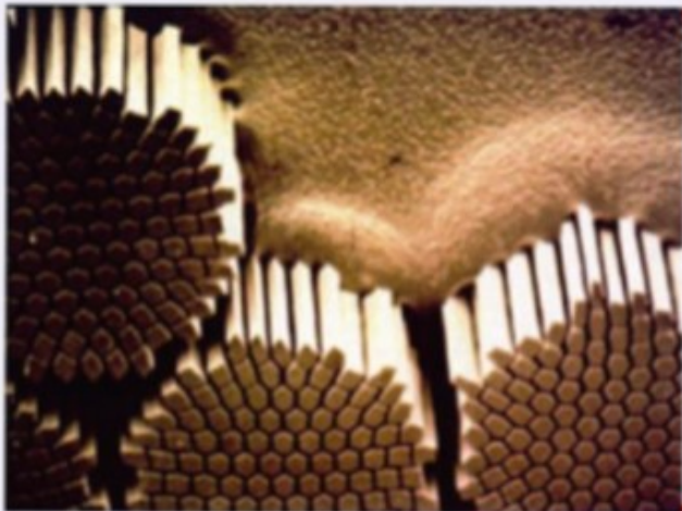
Fine filaments of Nb-Ti in a Cu matrix
