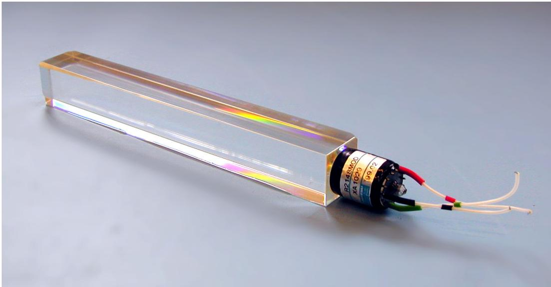
Electronic Calorimeter (ECAL)
