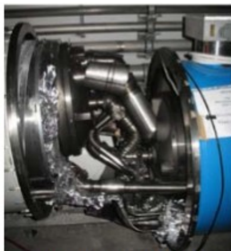
Damage at an LHC interconnect
