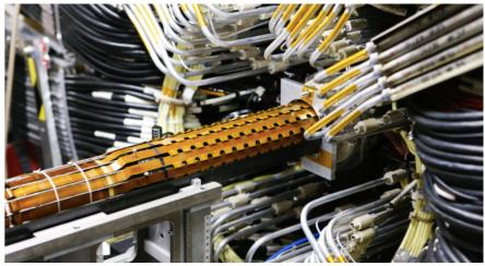
Very radiation tolerant detectors, first use in ATLAS Insertable B layer (IBL) 3.3 cm radius - improved impact parameter resolution
