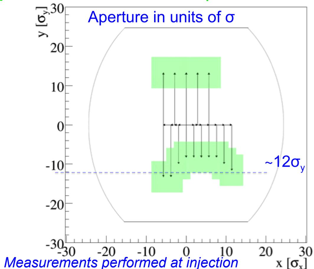
The aperture restriction seems to get worse between injection and top energy (and sometimes even at injection)! Current strategy: continue beam commissioning, monitor the behaviour of the ULO, and check with higher intensity beams.
