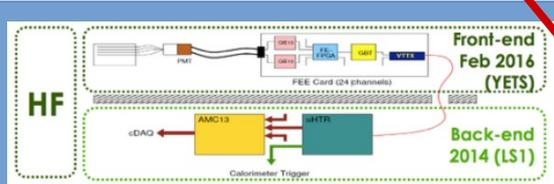
HF: switch to multi-anode PMTs and uTCA BE electronics
