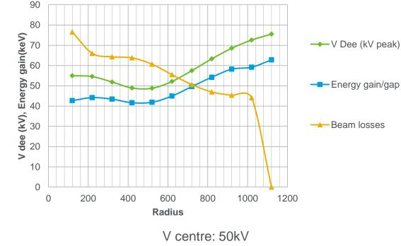
V centre: 50kV Power dissipated: 32.7kW N°of turns: 321
